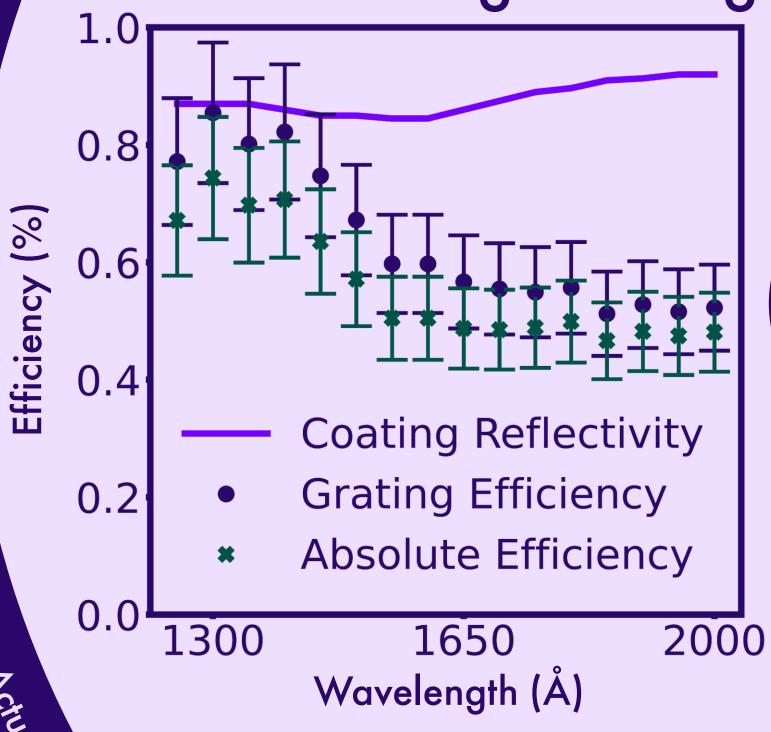
Actual Size of Mill St. Orinary. Xenon-enhanced lithium fluoride, an ultraviolet reflective coating developed at Goddard Space Flight Center, has been successfully applied to A88 mm diameter active area replica holographic
